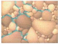
Water moving through tiny spaces in between sand particles or sandstone moves slower and allows for filtration of some contaminants.
